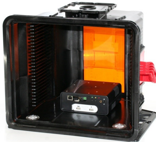
Figure 3: Measuring FOUP installation for the recognition of automated material handling anomalies
